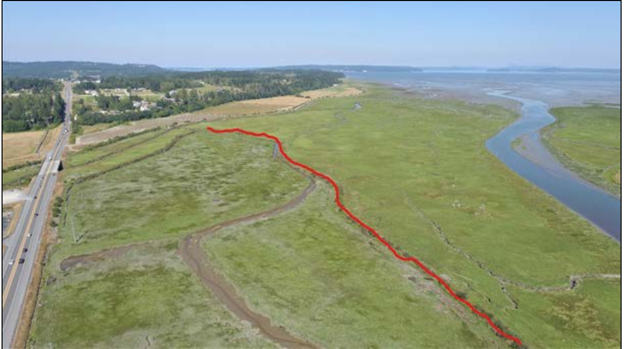
The North Leque project involves removing dike (shown in red) to improve access into marsh habitat for juvenile salmon - Photo by Desmul
