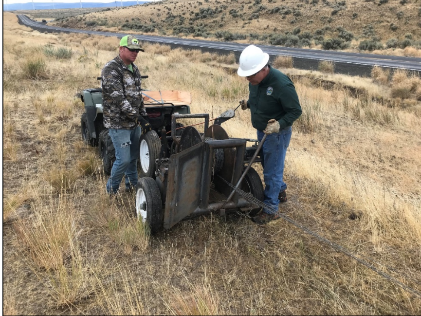
Motorized wire roller making short work of creating a spool of old barbed wire
