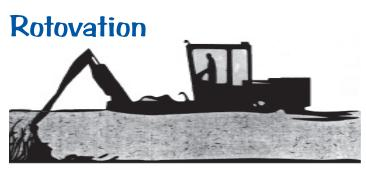
Rotovators are floating machines that use underwater rototiller-like blades to uproot aquatic plants. Rotovation is not an appropriate technique for addressing early infestations of aquatic noxious weeds.
