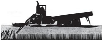
**Mechanical harvesters** are large floating machines that cut and collect aquatic plants. **Mechanical weed cutters** cut aquatic plants several feet below the water's surface but do not collect the plants while the machinery operates. Mechanical harvesters and/or cutters are not appropriate techniques to address early infestations of aquatic noxious weeds.
