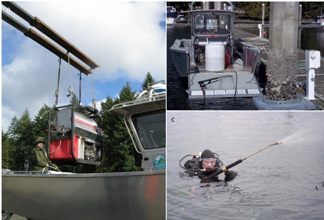
**Figure 9.** a) Loading a commercial pressure washer onto a landing craft vessel in preparation for acetic acid test spraying. b) Landing craft showing pressure washer, acetic acid container, and spray wand positioned near a test treatment piling. c) Diver about to submerge with diver-held spray wand.
