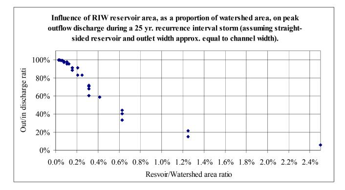
The general observation is that RIWs that impound wetlands less than about 0.2% of the area of the watershed are not likely to significantly affect the downstream flood peak flow in USGS region 2. As seen from the graph, out flow peak discharge is about 90% or more of the inflow. 0.2% of a one square mile watershed is about  $1\frac{1}{4}$  acre. On the other hand, RIWs with an area greater than 0.4% of the watershed may reduce peak flow by 50%.
