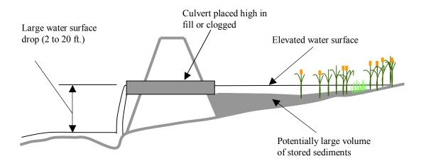
These three types of RIWs lead to different approaches to making decisions about the fate of the wetland and the type of crossing structure and hydraulic control. In the case of the independent type, the crossing itself has little to do with the wetland (although it should be constructed to accommodate the movement of the debris when it fails) and removing it might not change wetland conditions.
