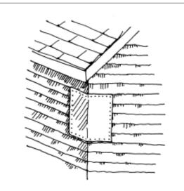
Figure 3. Raccoon access to rooftops can be eliminated by installing sheets of aluminum flashing, at least 3 feet square, around the corners of buildings.
