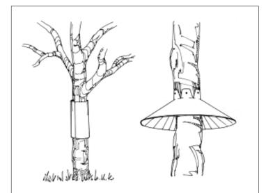
Figure 7. A raccoon guard can be secured around trees, pipes, posts, and other structures to keep raccoons from climbing. It can be made from a piece of aluminum flashing or sheet metal, held together with wire, nails, or screws, and painted to blend in.
