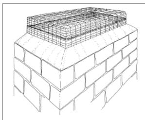
Figure 5. A commercially available chimney cap will prevent raccoons and other small animals from entering the chimney.
