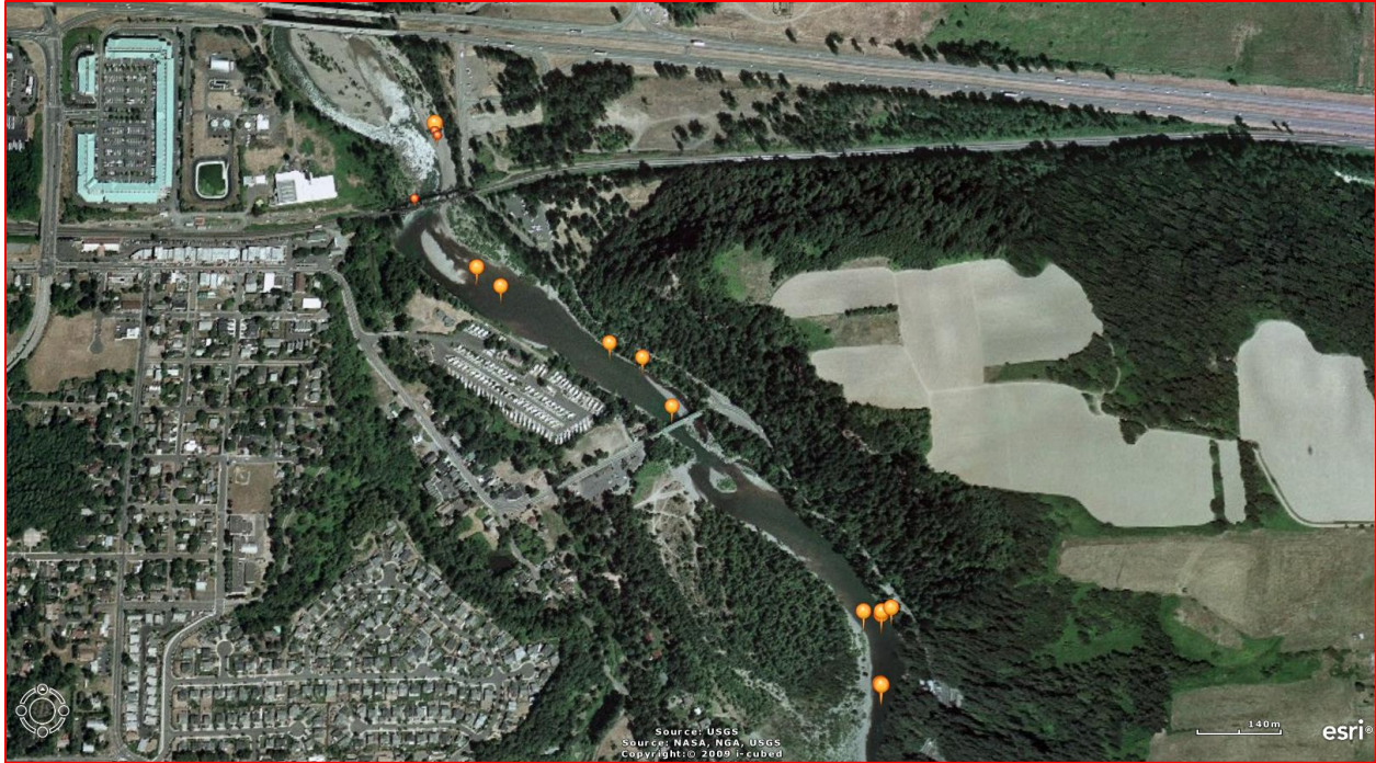
Figure 2. Distribution of sampling locations in the Sandy River, 27 January–2 June 2011. Red symbols indicate the locations of artificial substrate sets and orange symbols identify locations where ichthyoplankton tows were conducted.
