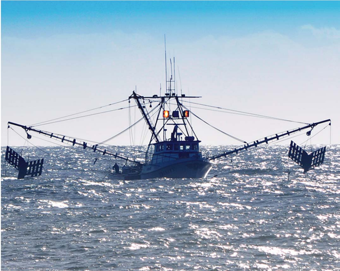
Shrimp boat with nets at the surface. Also pictured are the nets' mouth-spreading doors suspended from the vessel's outriggers.
