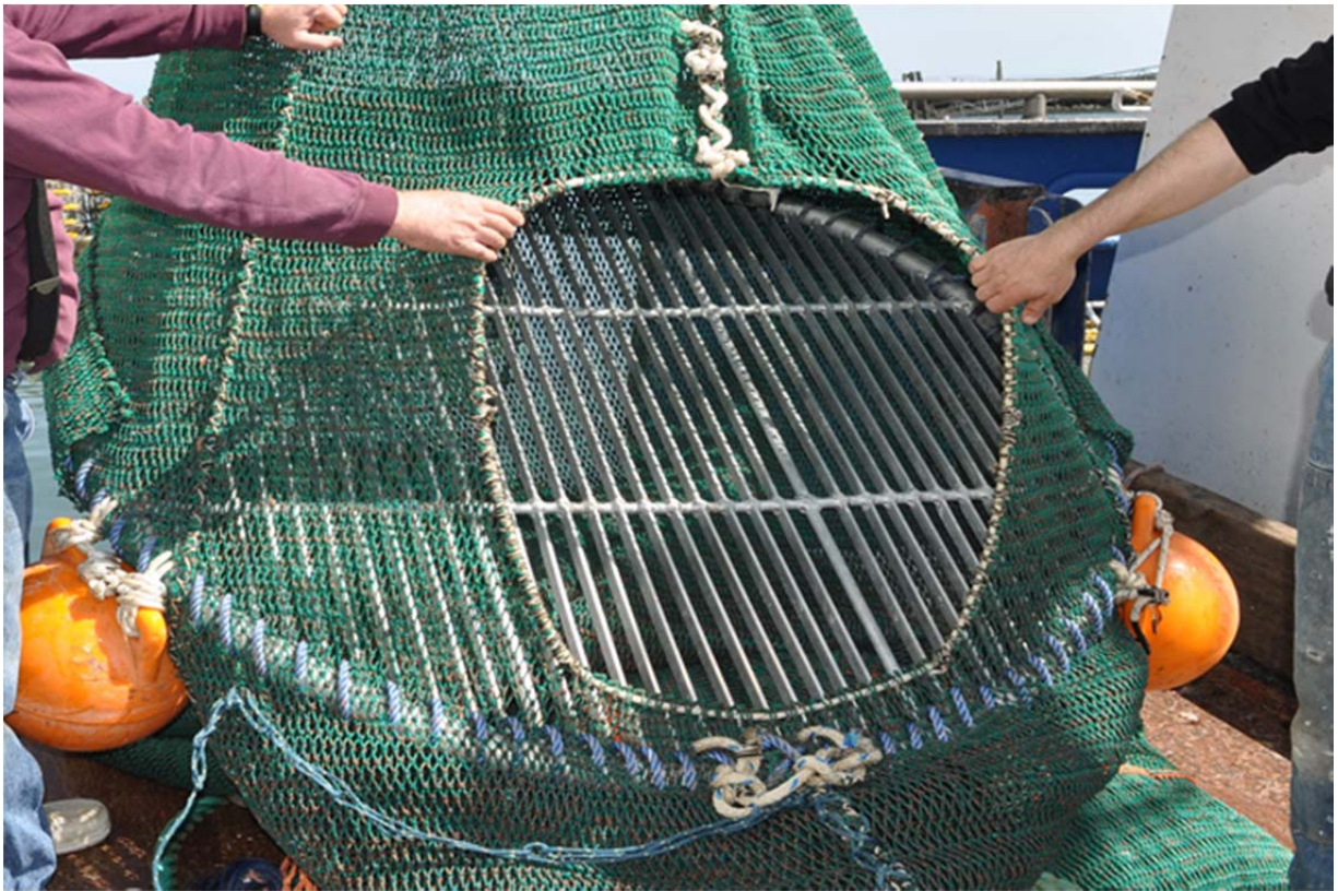
Excluder Panel shown through the escape hole on top of this net.
