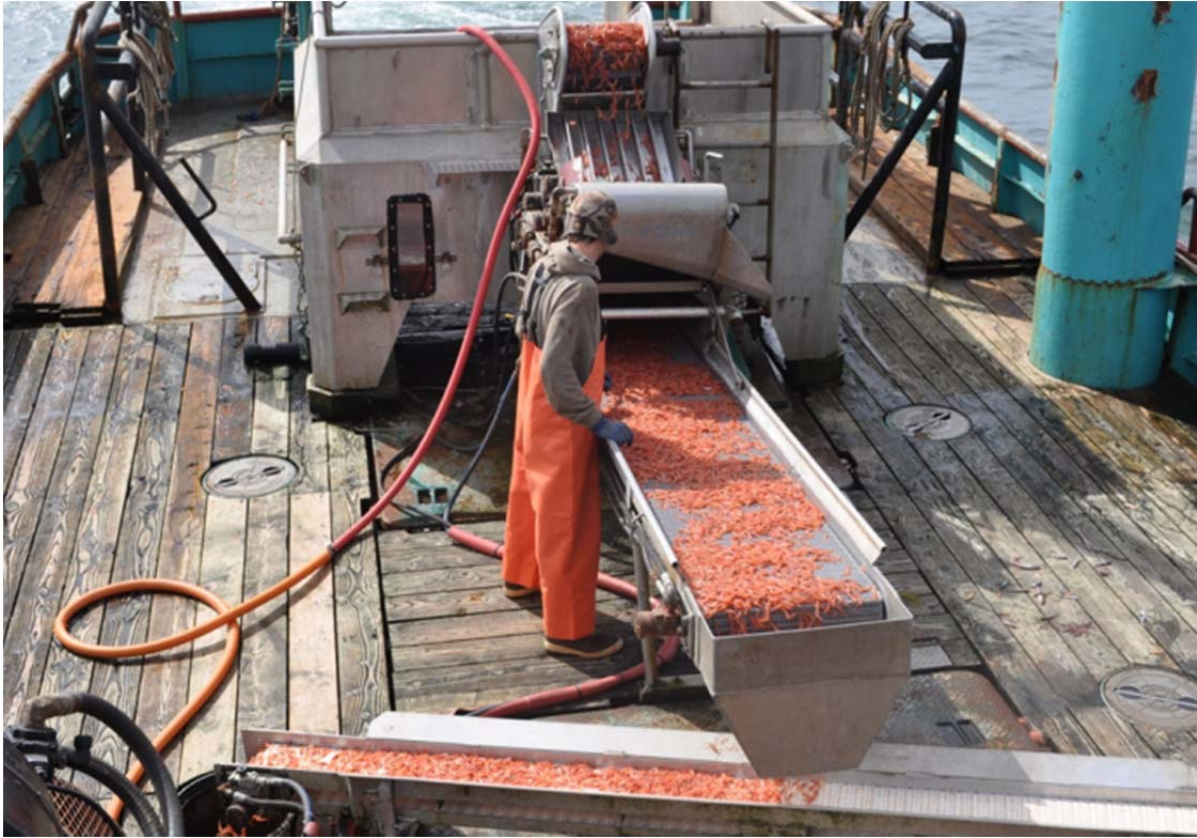
Conveyor belt moves shrimp from hopper to vessel hold. Crew positioned to remove bycatch.
