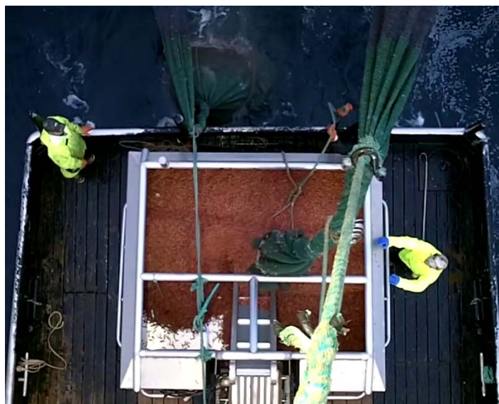
Shrimp being dumped from the codend of the net into the hopper on deck.
