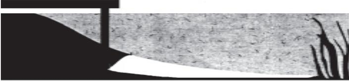
A bottom barrier covers the sediment like a blanket. By blocking light, it reduces the growth of aquatic plants.
