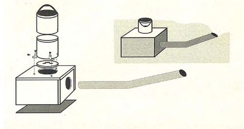
Figure 5. ABS design by Poulin et al. (2001) as used in Canada.
