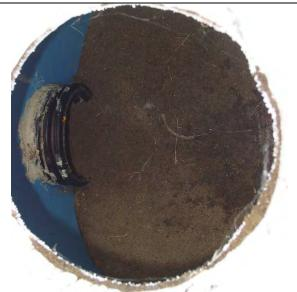
Figure 25. Looking down through pail at tunnel and collar into an installed burrow. Note the amount of adhesive placed around collar fitting; it is important that the collar stay firmly attached to the barrel chamber to prevent water and sand/dirt infiltration.
