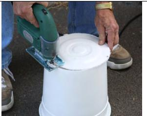
Figure 15. Use jigsaw to cut bottom out of one 2.5 gallon pail.
