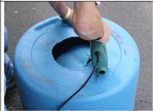
Figure 14. Use jigsaw to cut hole for pail to just slip about 1 in. into barrel.
