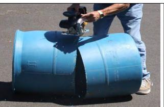
Figure 12. Cutting barrel in half with skillsaw.
