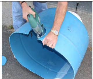
Figure 19. Cutting the 5.75 in. hole with jigsaw.
