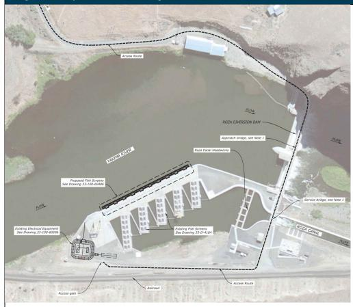
Modifications proposed to the screening area include saw-cutting the existing concrete headwalls and placing new concrete support structures for the slide gates and tracks associated with the new screens. Ten 8-foot diameter by 31.5-feet long stainless steel, wedge-wire T-screens would be installed in-river for this project.
