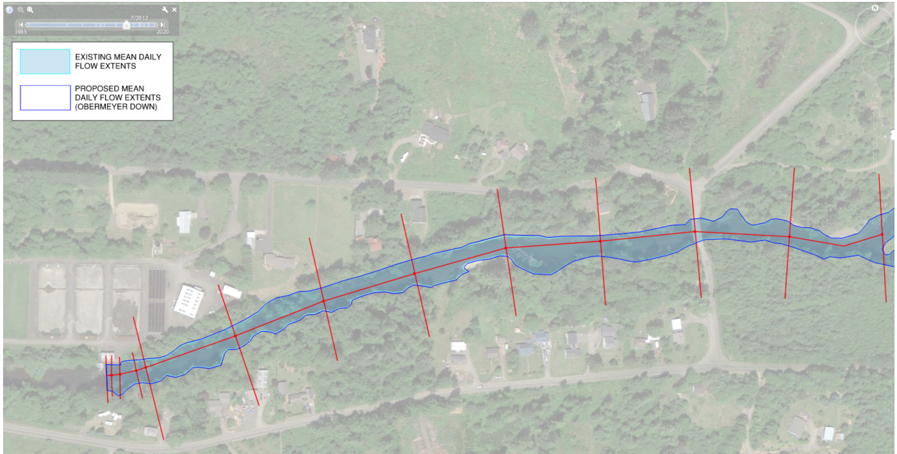
Figure 5-6. Plan View of Model Flood Extents Overlain on Aerial Photo of the Area (Mean Daily Flow)
