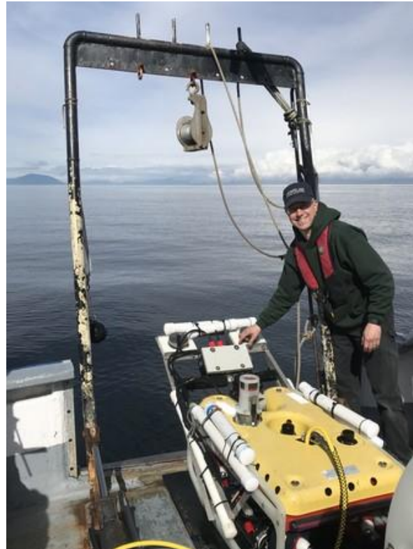
Seaeye Falcon, a Remotely Operated Vehicle in Marine Fish Science Unit.
