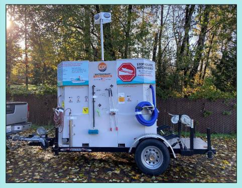
Trailer weight: 2,000 lbs (empty) Towing requirements: 2" ball hitch, max speed 55mph Prevent the spread of invasive species by remembering to **Clean, Drain, & Dry** your equipment!
