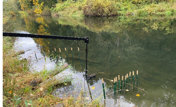
Sonar monitoring array installed on the Samish River. Photo by WDFW.
