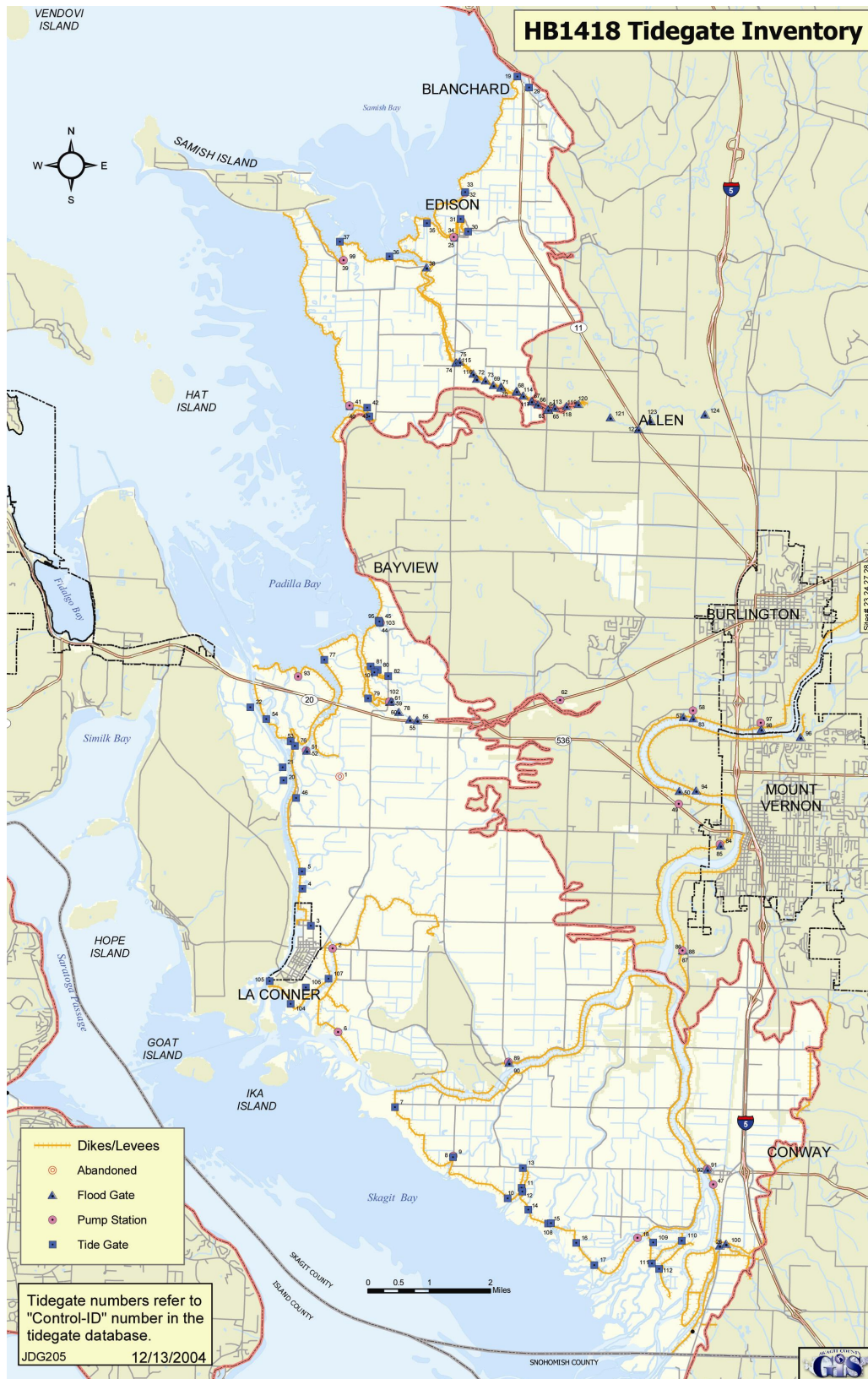
Figure 11. Tidegates, floodgates, and pump stations in WRIA 3 with a focus on those in the 1418 study area as outlined in red.
