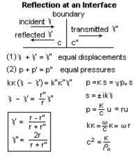
impedances r and r" of the two media. Finally, the simultaneous equations are easily solved for  $\xi$ ' and  $\xi$ " in terms of  $\xi$ , and the results appear in the box.
