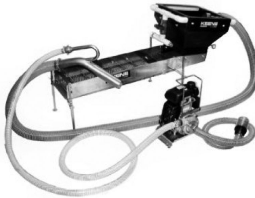
Figure 5: Power sluices/suction dredge combination
