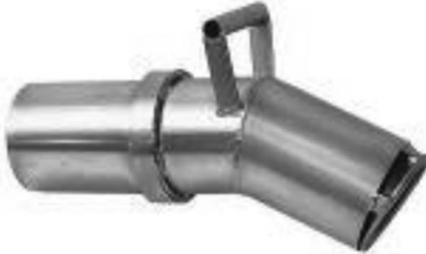
Figure 5: Dredge intake nozzle
