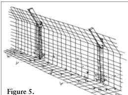
Fence extensions are required to keep coyotes from jumping over a 5-foot fence. Angle the top of a woven-wire fence out about 15 inches and completely around the fence. An effective fence extends below the surface, or has a wire apron in front of it to prevent digging.
