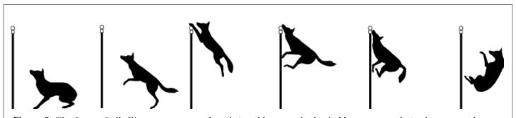
Figure 8. The Coyote Roller  $^{\text{TM}}$  prevents coyotes from being able to get the foothold necessary to hoist them over a fence.
