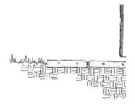
**a.**Lay large flat stones, concrete patio pavers, or 1/4-inch hardware cloth (held in place with stakes) on the surface of the soil next to a wall. The barrier forces coyotes to begin digging farther out and they will most likely give up in the process.
