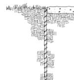
**c.** Excavate a 3 x 3 inch trench along the side of a wall, and hammer 2-foot lengths of 1/2-inch rebar, spaced a few inches apart, into the ground. Cover the tops with concrete or dirt.
