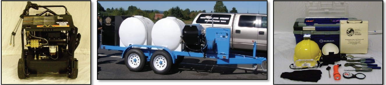
Figure 13. Regional (left) and trailerable (center) hot water pressure washers and personal safety equipment (right) used by WDFW personnel to decontaminate watercraft and other equipment.
