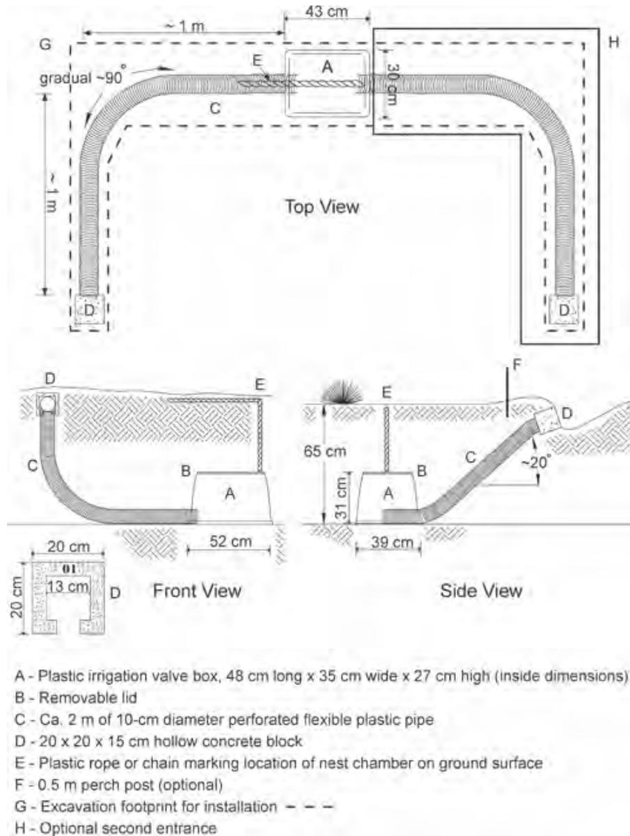
Figure 6. Artificial burrow system design by Barclay (2008).
