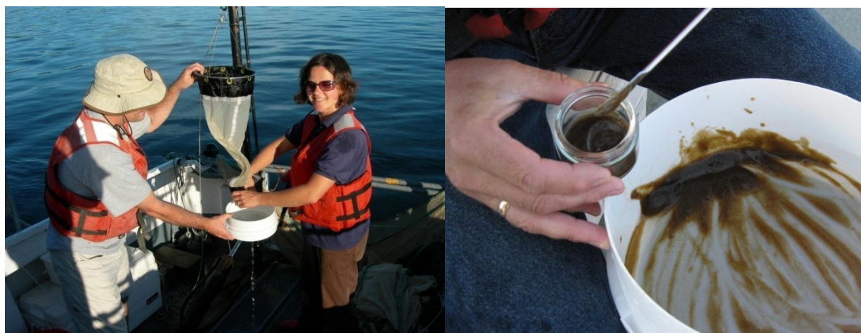
Figure 3. Conical plankton net and sieve (20 \mu\text{m} mesh pore size each) used to sample particulate organic matter (POM) and concentrate it into a paste.
