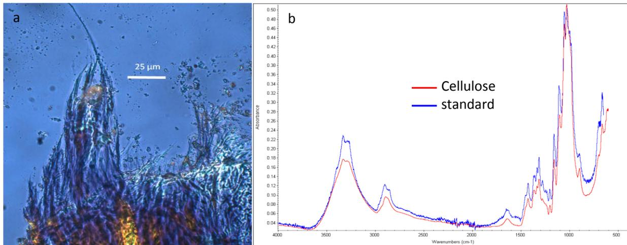
**Figure 11.** a) Optical microscope image of *Didemnum vexillum* from Shilshole Marina showing the fibrous structure remaining after protein digestion and bleaching. b) Attenuated total reflectance Fourier transform infrared (ATR-FTIR) spectroscopy comparison of processed *D. vexillum* from Shilshole Marina to a cellulose standard.
