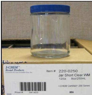
Figure 8 Pre-cleaned Series 200 I-Chem sample jar.
