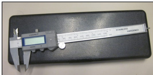
Figure 7 Stainless steel caliper with digital readout to 0.01mm.
