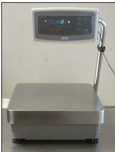
Figure 10 20-kg capacity bench scale for weighing large specimens
