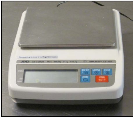
Figure 11 Six (6)-kg capacity bench scale for weighing small specimens.
