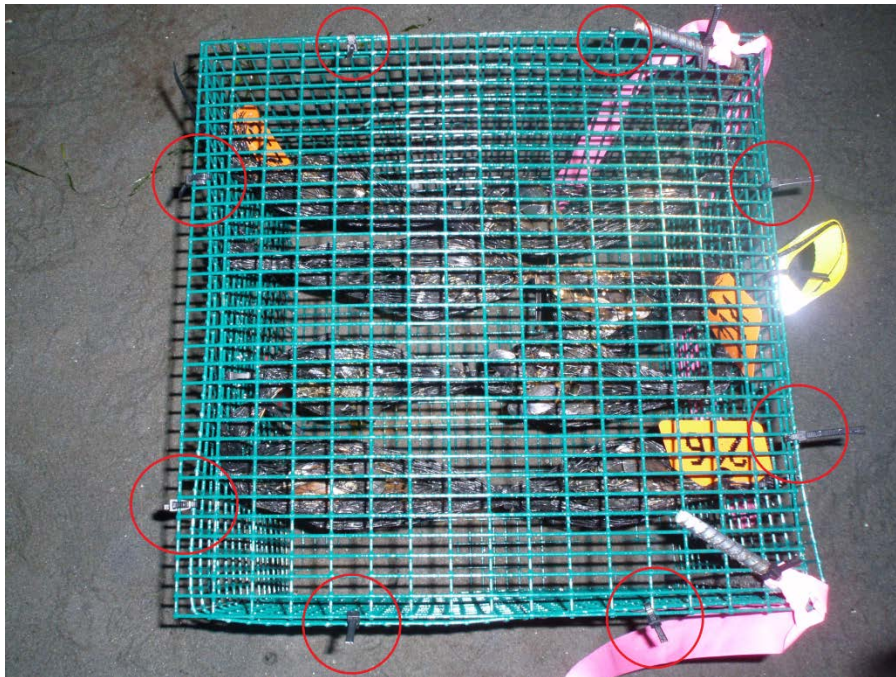
Figure 6. Anti-predator cage lid secured in place with at least two 8-inch cable ties per edge (red circles).
