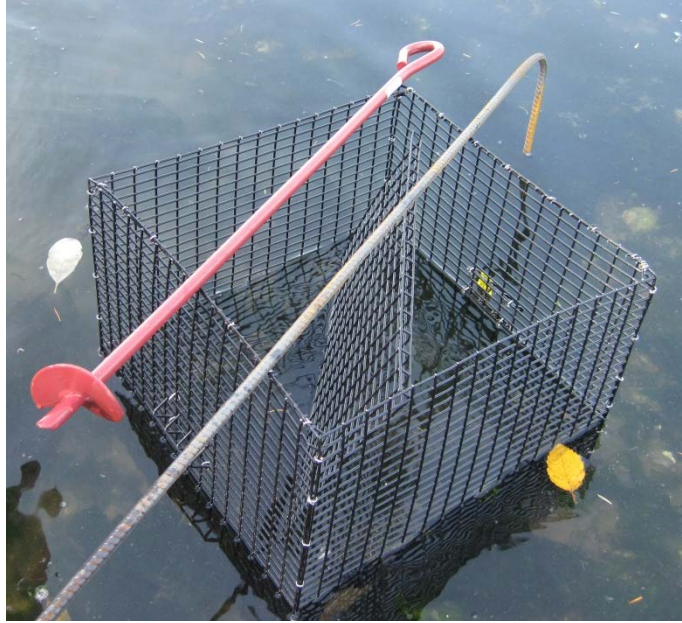
Figure 4. Anti-predator mussel monitoring cage (lid shown inside cage) with 30-inch screw anchor and bent-tip rebar stake.
