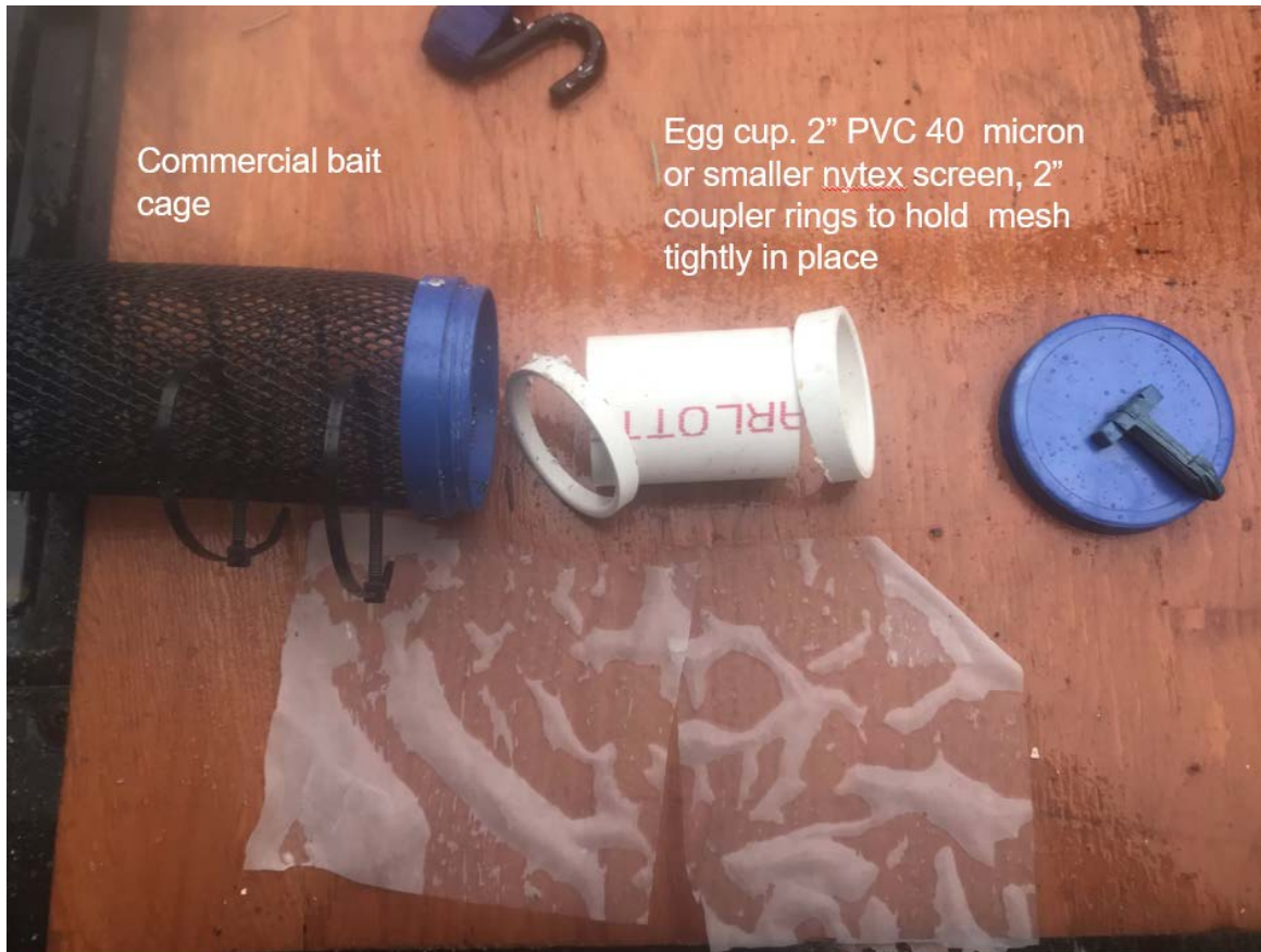
Figure 1: Photo of embryo cage materials including commercially available bait cage, two-inch PVC pipe sections, coupling rings, and 40 micron Nitex mesh.
