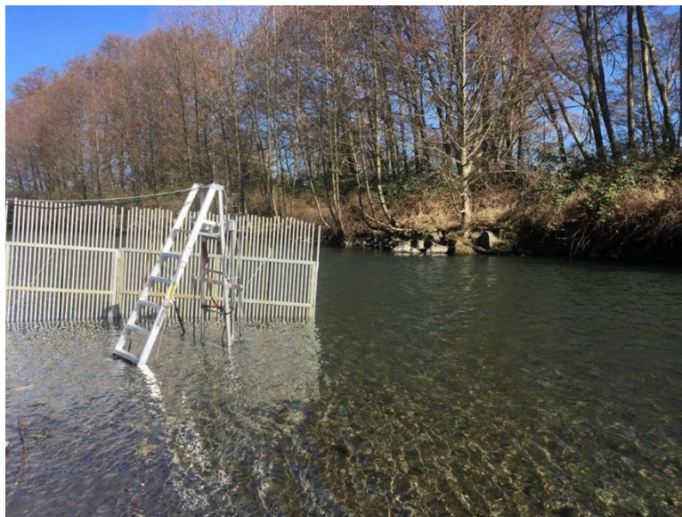
Figure 3.3: SONAR unit deployment via a pole mount and ladder system in the Dungeness River in 2018.
