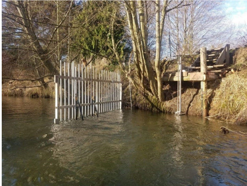
Figure 3.4: SONAR unit deployment via a pole mount and platform in the Dungeness River in 2020. Picket weir is the upstream picket weir.
