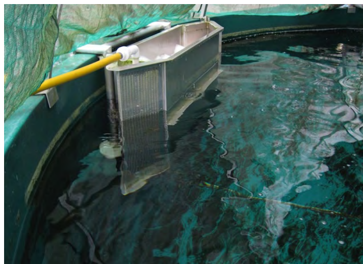
Figure 7-5. Airlift System in a Circular Tank.
