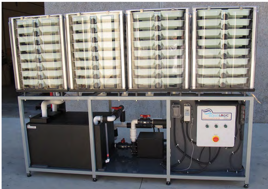
Figure 7-4. An Example of a Recirculating Egg Incubation System Designed by Aqua Logic that includes 4 half-stacks, chiller, UV disinfection, water mixing sump, pump, and controls.
