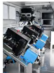
Figure 4. Computer controlled AutoFish System inside trailer containing a sorter and six marking and tagging lines. Adipose fins are clipped via black mechanisms and then CWT inserted using blue injectors. Source: Northwest Marine Technology
