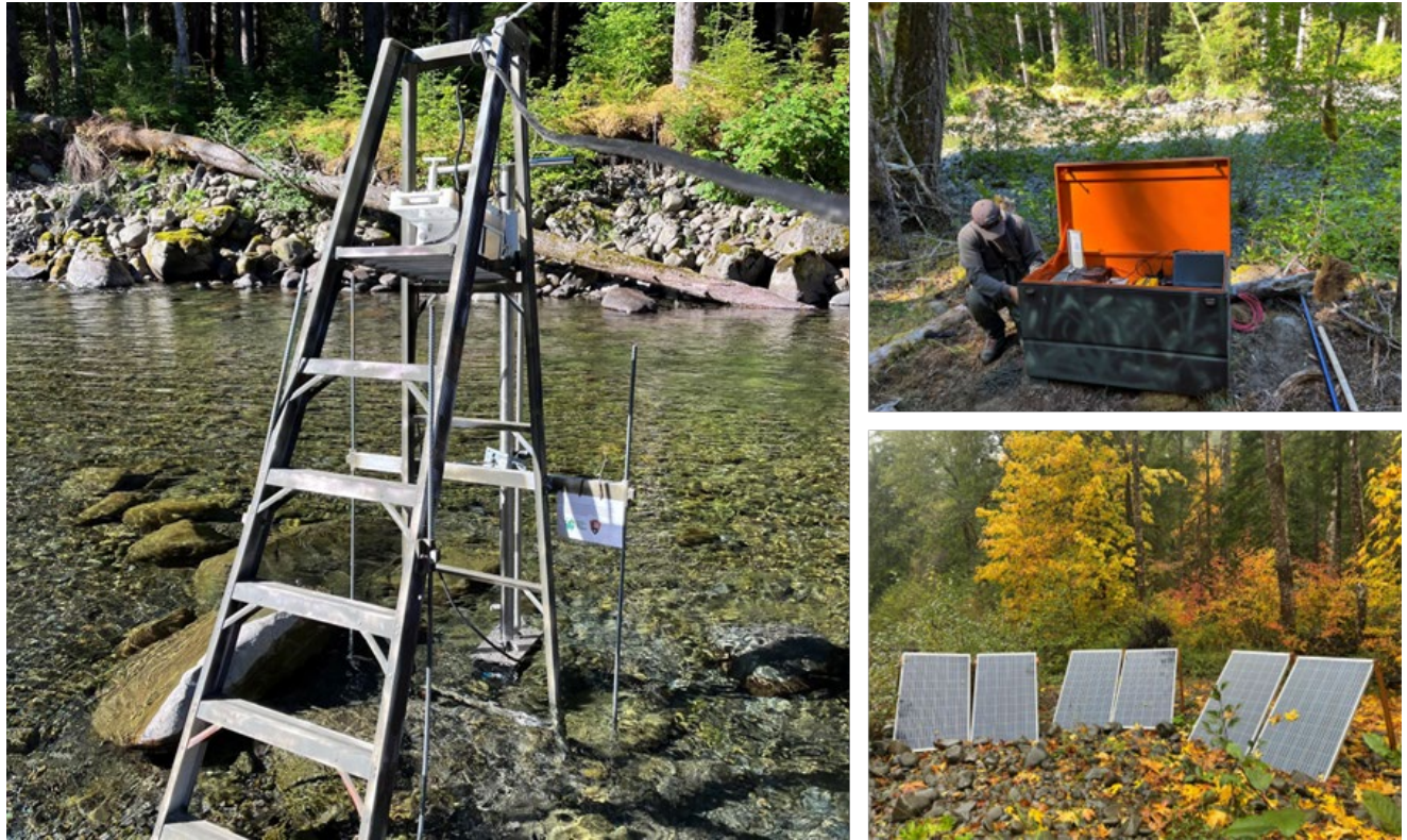
Figure 2. Clockwise from top left: SONAR mounted on an aluminum ladder upstream of the Salmon Cascades on the Sol Duc River at river mile (RM) 56.8, jobsite storage box housing the batteries, inverter, and laptop, and solar panels used to power the ARIS Explorer 1800 SONAR unit.
