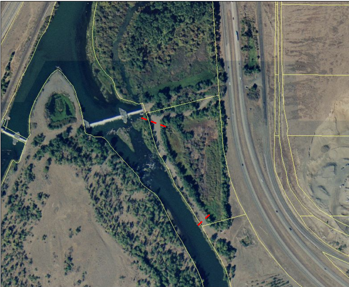
Figure 2. This aerial photo shows the project location in relation to Wapato Dam (east) and the red dotted lines indicate the proposed inlet and outlet locations (areas of excavation) to establish perennial flow through this parcel.
