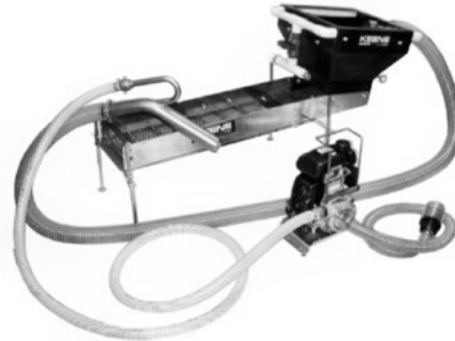
Figure 5: Power sluice/suction dredge combination
