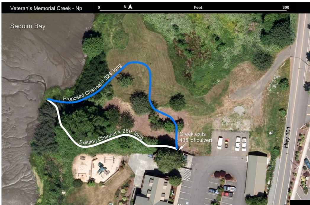
FIGURE 4: SITE IMAGE SHOWING THE LOCATION OF PROPOSED RESTORED STREAM CHANNEL AND THE EXISTING DEVELOPMENT OF THE SITE
