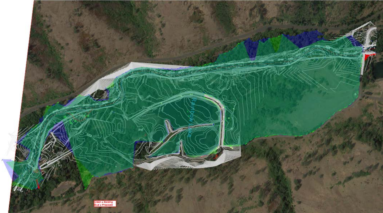
Figure 4. 100-year inundation map. Bright green areas are existing inundation. Dark blue areas are proposed conditions inundation. Aqua areas are overlap of existing and proposed conditions.
